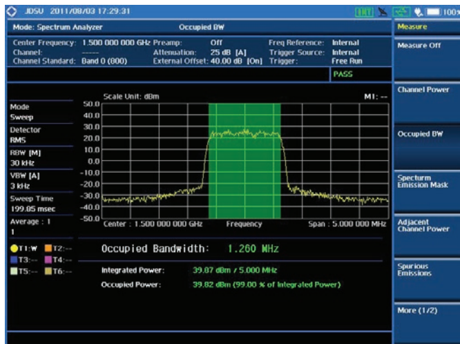
RF analysis — Occupied Bandwidth
