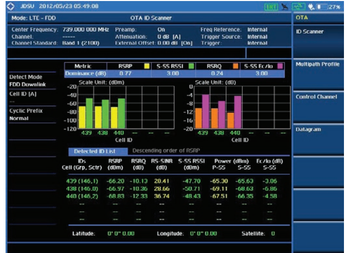
OTA analysis — ID (Channel Scanner)
