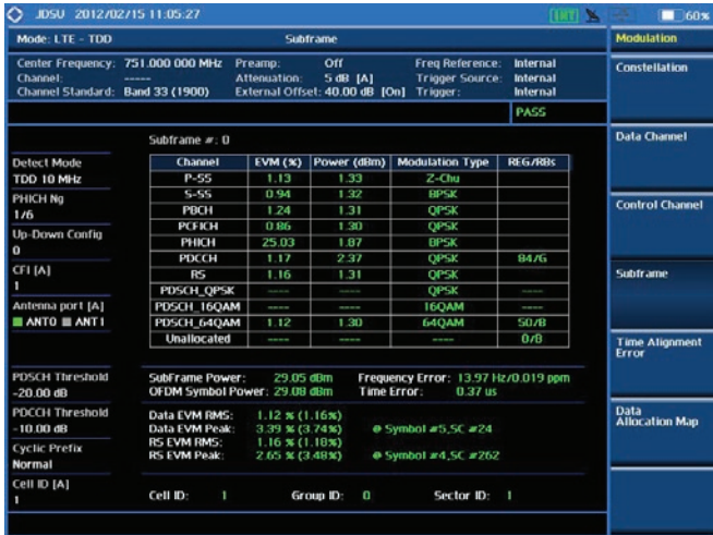
Modulation analysis — Subframe
