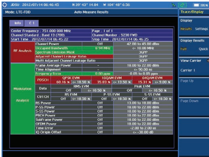
RF and Modulation analysis — Auto Measure
