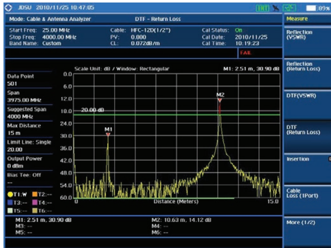
Cable and antenna test — Distance to Fault
