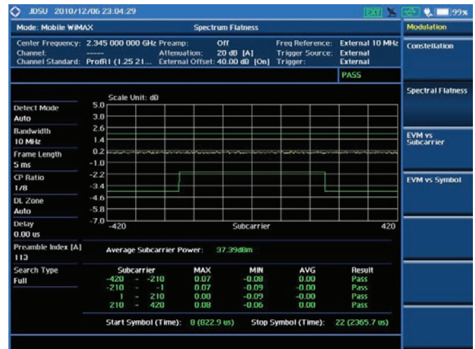
Modulation analysis — Spectral Flatness
