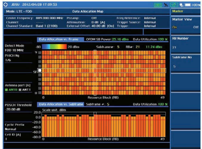
Modulation analysis — Data Allocation Map
