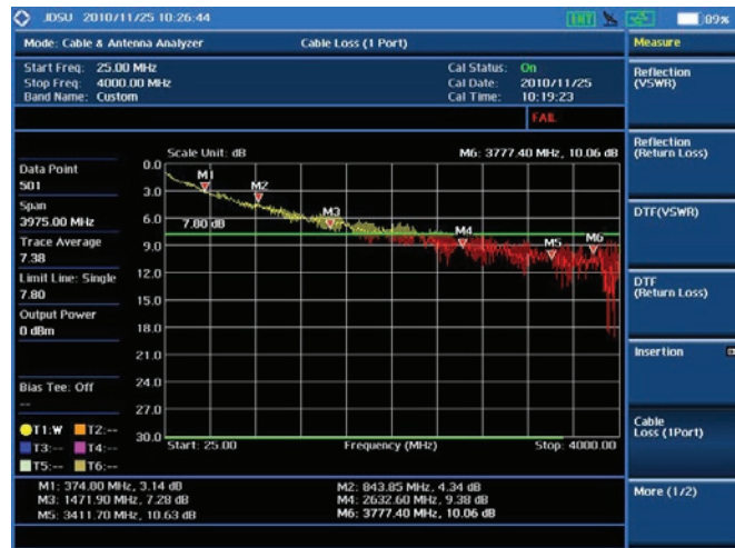
Cable and antenna test — Cable Loss
