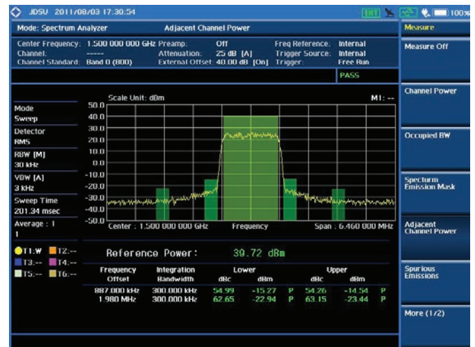
RF analysis — Adjacent Channel Power
