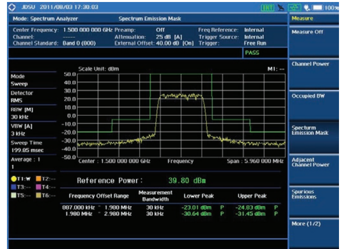
RF analysis — Spectrum Emission Mask
