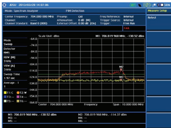
RF test — PIM Detection
