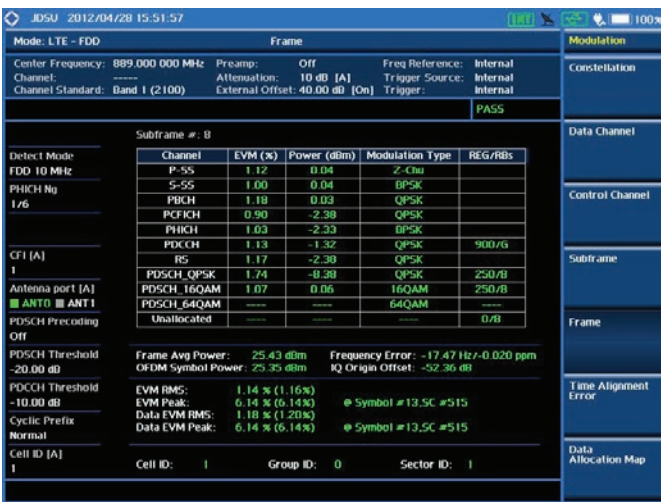
Modulation analysis — Frame
