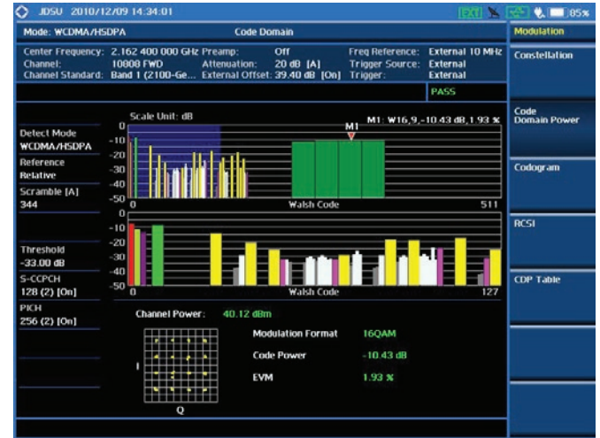
Modulation analysis — Code Domain Power
