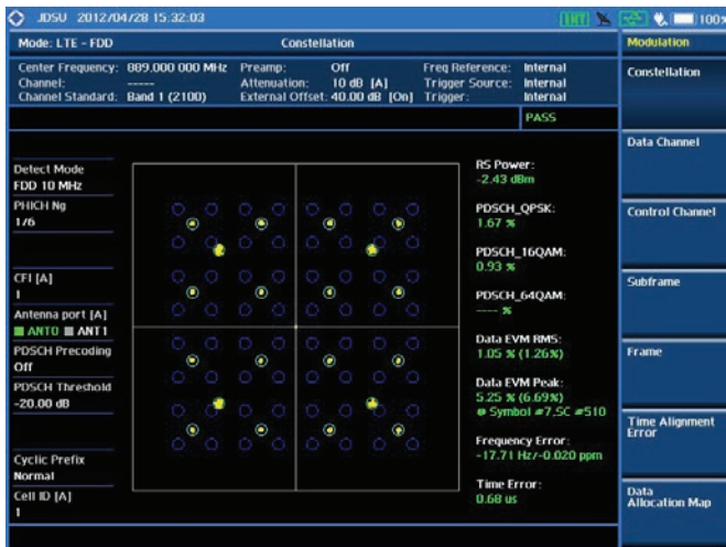
Modulation analysis — Data Constellation
