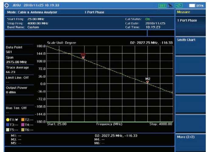
Cable and antenna test — 1-Port Phase
