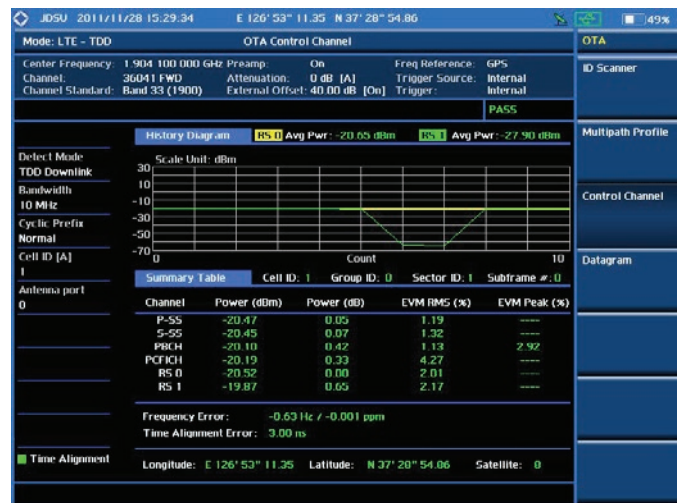
OTA analysis — Control Channels
