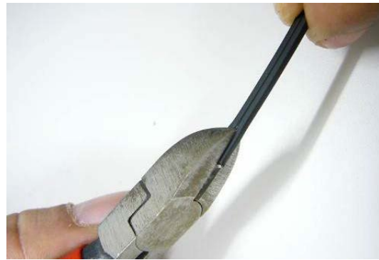
4: Make a slit along the groove of the cable sheath using nippers.
